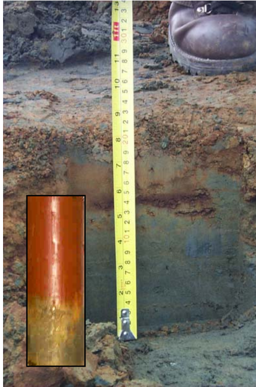
Figure 2: Field example of sludge layered over tailings. Inset shows a core of a sludge over tailings disposal scenario.
